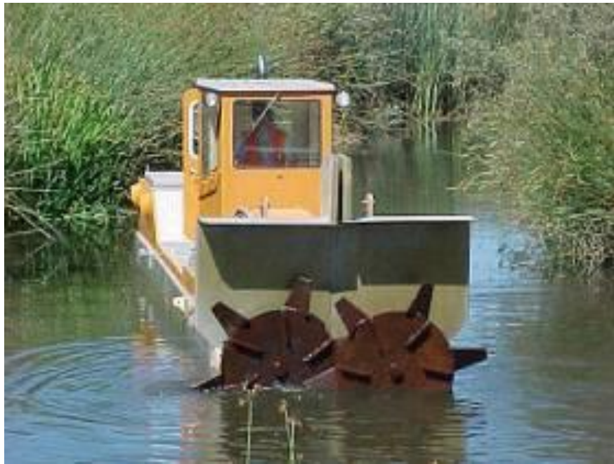
Figure 2. Photo of Cookie Cutter vegetation shredder, similar to one used on Bayou DeSiard in 1981.
