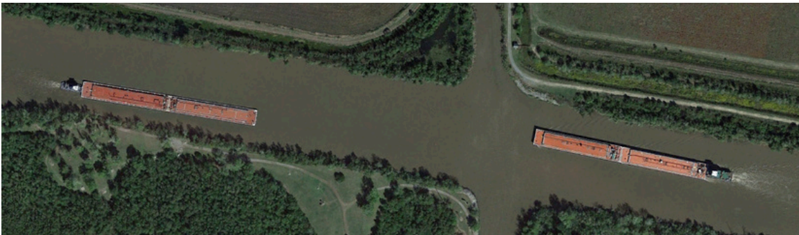
Figure 7. Barge traffic on the GIWW can be seen in this Google Earth imagery from 2012 and is a key contributor to shoreline erosion.
