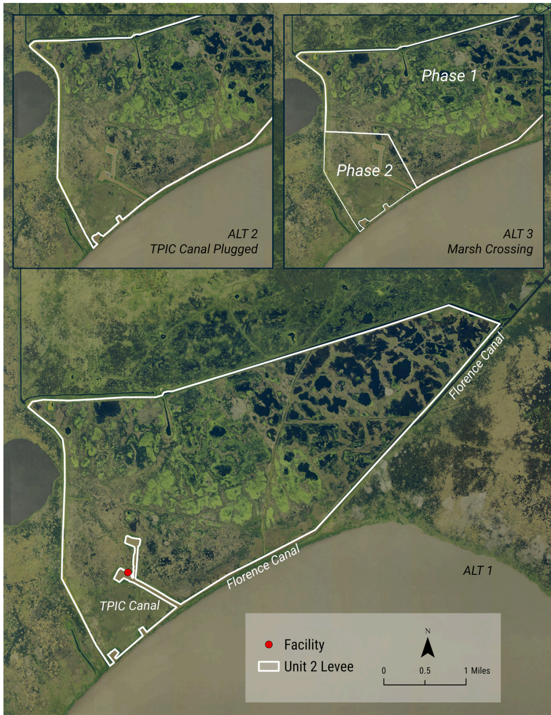
Figure 11. Three Unit 2 levee restoration alternatives are depicted in this figure. Alternative 1 involves repairing the levee within its existing footprint, as illustrated in the bottom map. In Alternative 2, at the top, left, the TPIC canal is plugged at the Florence Canal. Alternative 3, at the top, right, includes two phases. In Phase One, a new levee is built across the marsh, bypassing the TPIC canal entirely. In phase two, the remaining area of the Unit 2 levee is repaired after oil and gas extraction has ceased.
