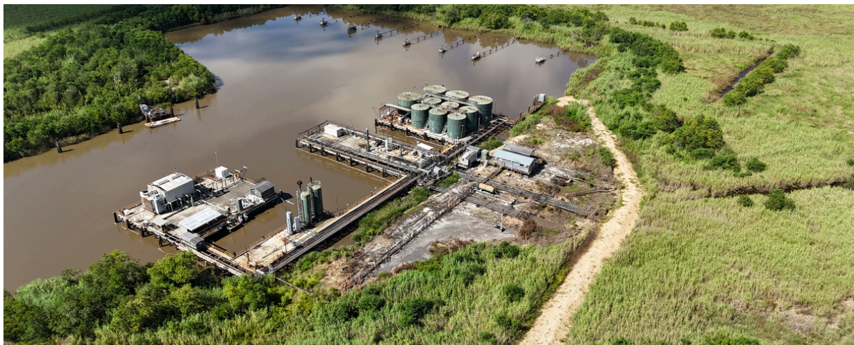
Figure 10. A portion of the TPIC facility is shown in this image with associated pipelines running along the ground and oil and gas infrastructure in the location canal - all of which complicates restoration and maintenance of the Unit 2 levee.
