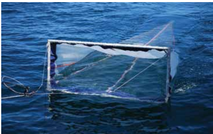
The SEAMAP Plankton cruise utilizes two different net types. Neuston nets (left) are towed continuously at the surface, while Bongo nets (right) are lowered to depth and towed slowly as they are lifted through the water column. Both provide information on the occurrence, abundance, and distribution of eggs, larvae, and juvenile fishes and invertebrates.
