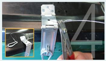
**4** To lock can, place clip, quick snap or carabiner through latch plate after hasp is in place. Use chain, wire or string as pictured to avoid losing or misplacing clips, quick snaps or carabiners.
