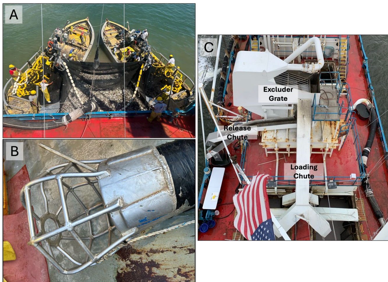
Figure 2. (A) Purse boats alongside the sampling vessel with catch being pumped from the net via the large suction hose. (B) The hose cage used as a bycatch reduction device to prevent large bycatch from being entrained within the hose and pump. (C) Standard vessel layout showing the loading and release chutes and the fish exclude grate used as a secondary bycatch excluder device.
