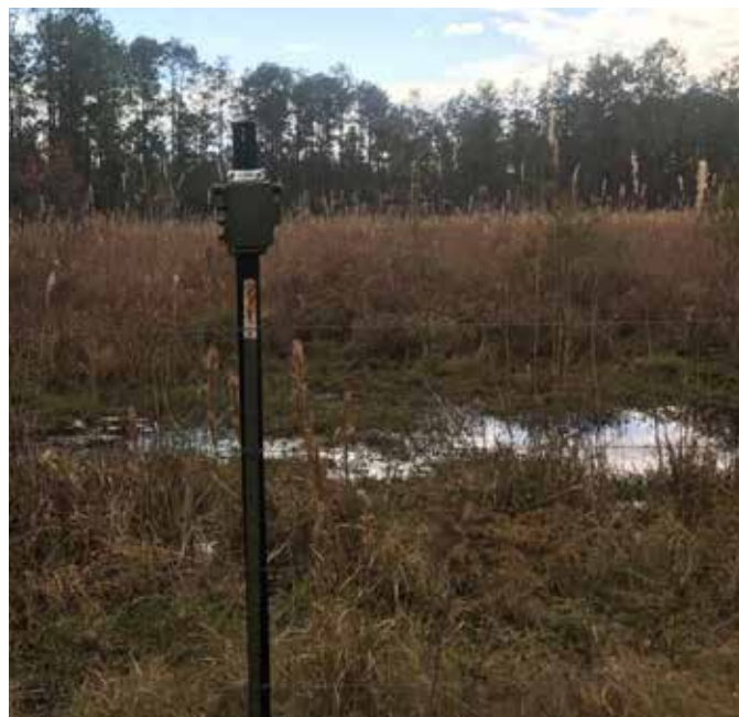
Automated Recording Units: An automated recording unit (ARU) used to record calling frogs.
