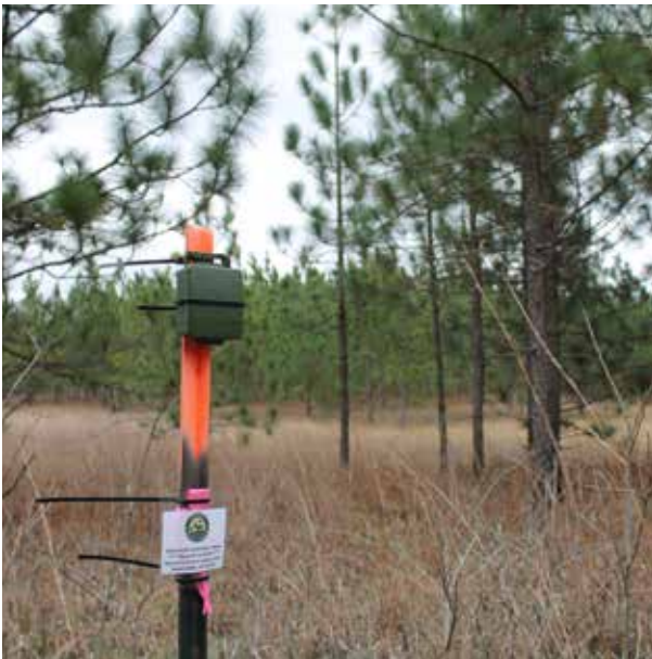
(LEFT) Autonomous Recording Units (ARU) : An autonomous recording unit used to record bird vocalizations. (RIGHT) Other surveys : The LDWF Ornithologist conducts a survey for Whimbrel.
