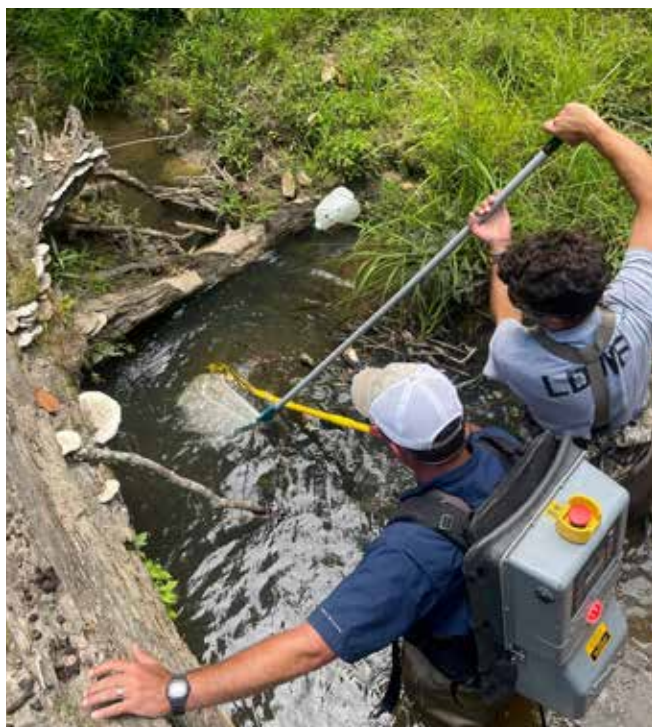
Electrofishing: LDWF staff use a backpack electroshocker (ABOVE) and electroshocking from a boat (BELOW) to survey for inland fishes.
