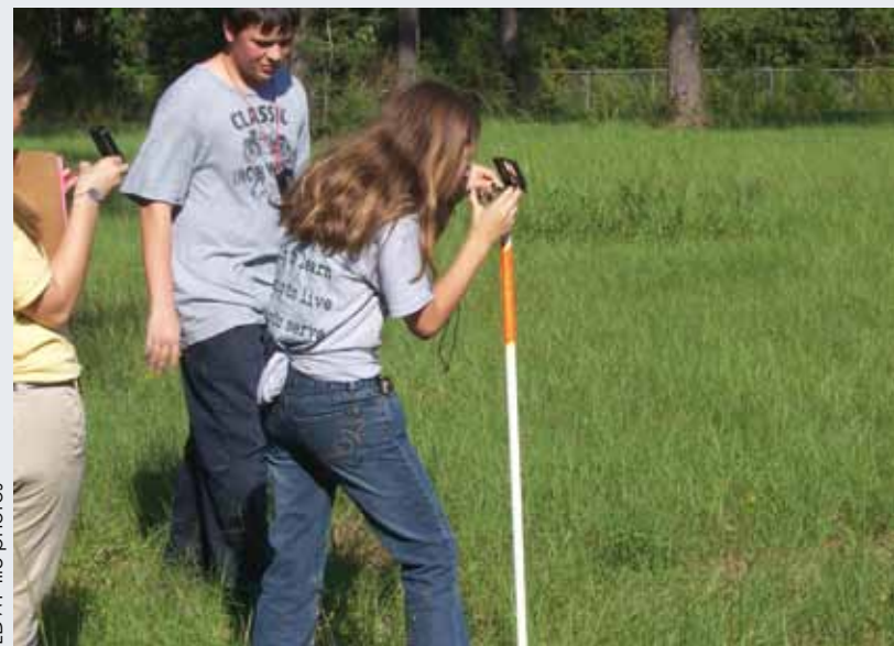
Compass and pacing. Students determine bearings and pace distances on the compass and pacing course.
